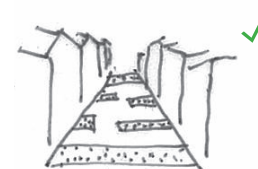
Variety of surface finishes and materials and clear threshold between lane and adjoining street
