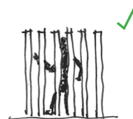
Full height semi-permeable fence providing both privacy and connection to lane. (40-50% permeability)
